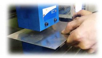
3. PLACE MATERIAL UNDER TOOL AND PERFORM TEST PUNCH.
