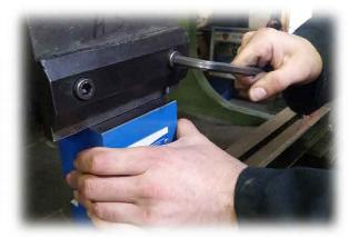
1. INSTALL TOOL IN PRESS, ADJUSTING FOR MAXIMUM CLEARANCE BETWEEN PUNCH AND DIE CUTTING BLADES.
