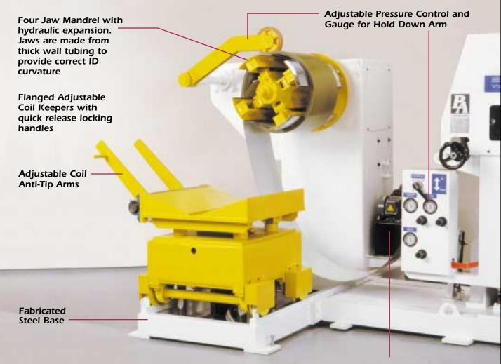
Self-contained Hydraulic System for mandrel expansion and coil car lift & travel
