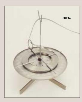
These reels offer an efficient and safe way to handle horizontal pay-off problems. Off center loading, which is characteristic of pan reels, is not a problem for P/A. This reel is designed with a combination of a Timken tapered roller bearing and radial ball bearing housed in a rugged, cast iron hub. This dual bearing design permits easy and safe coil loading by eliminating the "tip-over" threat. Centering the coil on the platen is no longer necessary.
