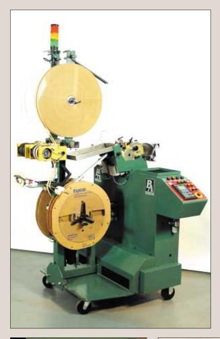
P/A Automatic Winding Equipment incorporates high-quality design and components to make these units virtually maintenance free. Welded steel construction provides long term rigidity and stability while lockable casters provide ease of movement and positioning.
