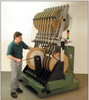
The same-side load and unload feature of this Automated Winder helps to improve material handling in tightly packed press shop environments.
