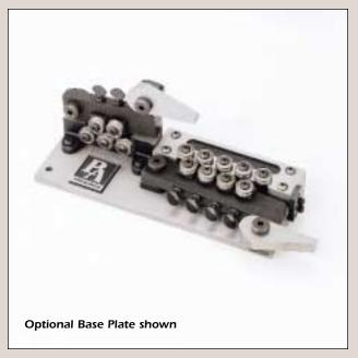
The Dual Plane P/A Wire Straightener was originally designed for the rugged conditions of wire mills. The shielded, anti-friction ball bearings have "V" grooves ground into the hardened outer races. All rolls are prelubricated. A spring loaded feature compensates for wire irregularities. Rolls are adjusted by a thumb screw and locknut.
