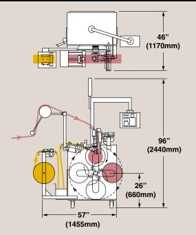
The LW 15-4P is a fully automatic traverse winder equipped with a universal material feeding and guiding head. The winder automatically inserts the strip into the empty spool and fills the spool until the preset number of terminals is reached.
