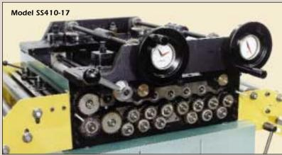
These powered straighteners are designed specifically for thin and high tensile strength materials such as silicon steel for motor laminations and stainless steel or titanium for medical instruments. Solid cast frames ensure precise roll parallelism for optimum straightening results.
