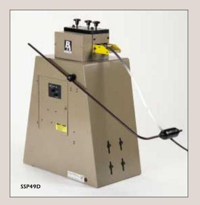
This eleven roll straightener (nine straightening rolls) is very well suited for phosphorous bronze and stainless steel, or other types of difficult to straighten material. It's recommended for applications in which the strip must be absolutely flat before stamping, such as with electrical switch elements and contacts.
