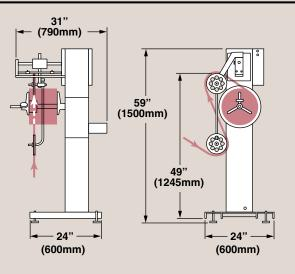
The LW Semi-Manual Layer Winder is a basic machine designed to wind material strips in a traversing, side-to-side manner. Once preset for a winding range, this machine will continue to fill each new reel until it is interrupted by an operator, or a tight loop condition.
