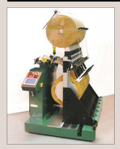
Lower your Man-to-Machine Ratios or run unattended with up to 10 reels of Automated Winding.
