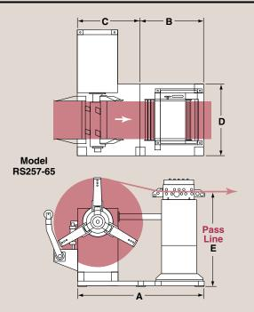
When floor space is at a premium, consider this Space Saver design by the innovative P/A engineering team. The Stock Reel is equipped with an adjustable caliper disc brake to provide the right amount of back tension. The DC drive Stock Straightener is offset for easy loading. The loop-sensing arm automatically adjusts material payout speed to press requirements. These units are equipped with entrance cascade and exit pinch rolls. Specify left-to-right or right-to-left stock travel.
