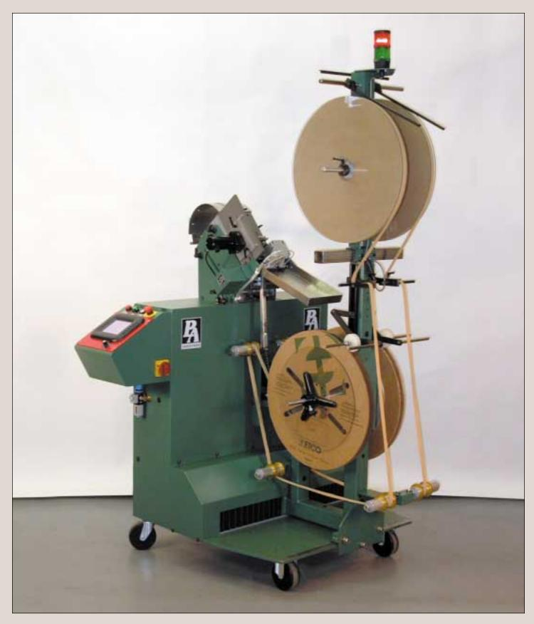
Increased productivity is the motivation behind the introduction of entry-level automation. These compact, high-speed units perform automated reel changes based on a pre-programmed number of parts per pancake reel without stopping the press. This makes them ideally suited for continuous stamping, plating and molding operations.
