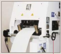
Handwheel, self-centering material roller, edge guides and separate stock position adjustment
