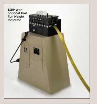
The advantages of these straighteners are immediately obvious. The Flip Top makes strip loading easy. Simply swing open the head, feed in the strip, close and tighten. Single-point adjustment for each roll ensures a precise setting and eliminates the cambering often caused by nonparallel rolls.
