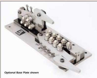
As the wire is drawn through the P/A Wire Straightener, each plane of "V" groove rolls removes the natural curve of the coil, neutralizing the tendency to kink, twist, whip, or distort. The first plane of rolls must do more work, which allows a lesser number of rolls on the second plane. This reduces the amount of pulling power required.
