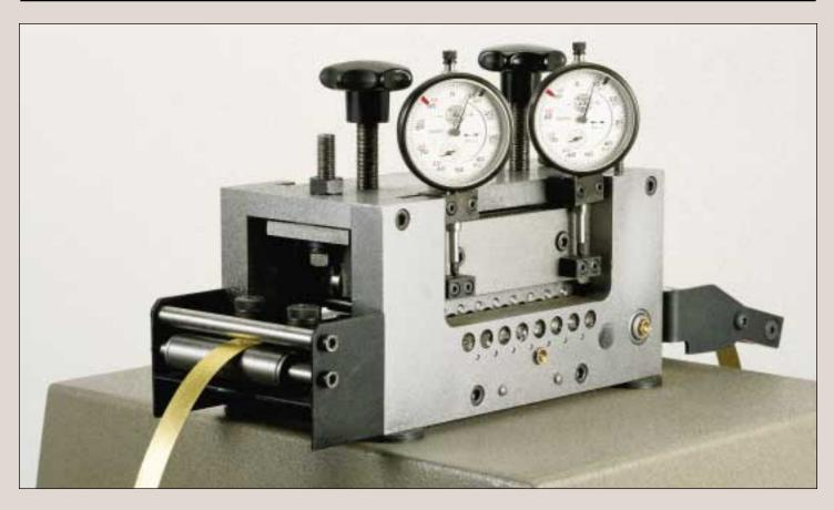
The P/A Ultra Precision Stock Straightener was designed with the electronics stamper in mind, especially those using exotic coppers or clad materials in their operations. A very unique design employs seventeen straightening rolls which are backed up by roller bearings in a precision machined steel body.
