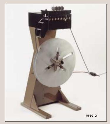
The P/A Flip Top Reel Straightener is a combination of the Flip Top Stock Straightener head and payoff reel for easy material loading and maintenance. Available in two configurations, these models will minimize the use of precious floor space.
