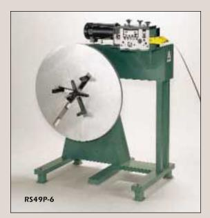
At last, a precision reel straightener that not only saves floor space, but is also easy to load. Nine different models are available with material widths up to 6 inch (150mm) and coil weights up to 600 lbs. (272 Kg). This unit should be of special interest to the electronic stamping industry for processing hard to straighten materials, such as beryllium copper, phosphorous bronze and brass.
