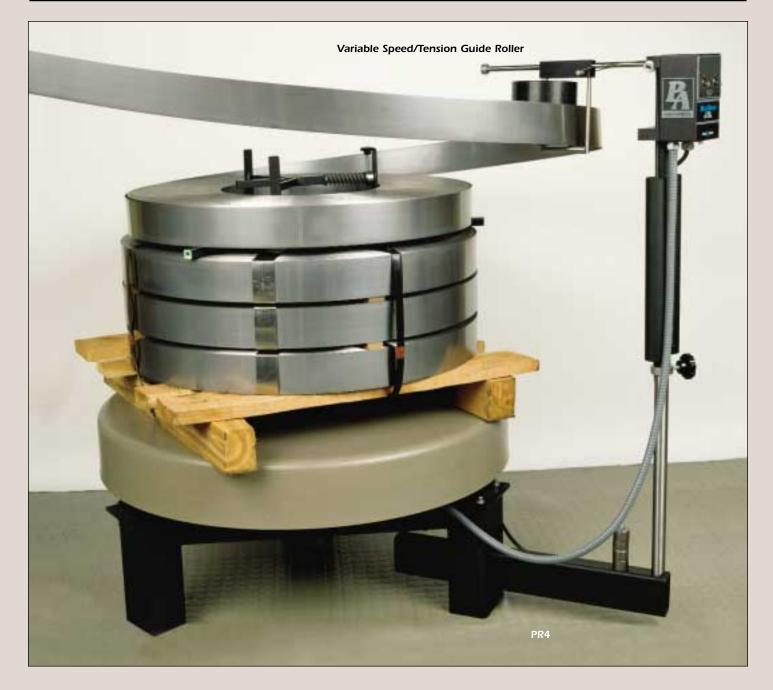
The Palletizer was designed to pay off pre-stacked coils of material one coil at a time. This simple, yet innovative, design effectively reduces the risk of injury to operators and damage to material by eliminating the handling of individual coils.
