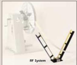
of the Reel or Straightener to maintain a constant loop. The RF is not susceptible to ultrasonic interference which makes it an attractive alternative to sonar sensing systems.
