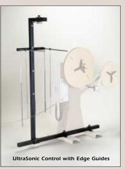
control eliminates signal drift, while the coded sound bursts reject interfering sound waves.
