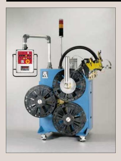
Material Feeding Assembly The LW 24-3 Traverse Layer Winder is a 24-inch, 3 station, automatic material winder capable of continuous operation when assisted by an operator.
