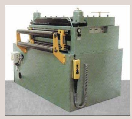
The Magnum Heavy Duty Straighteners are built to meet requirements for removing coil set from thicker, wider material. They have been designed to compliment the P/A Magnum Servo Roll Feeds.
