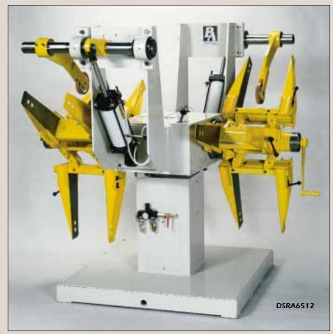
These Dual Reels use the same rugged construction as that of the Single Reels. The motorized versions have two proportional speed DC or AC motors, one for each spindle. Each drive motor uses a gear reducer with torque limiter for additional gearbox protection.
