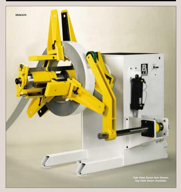
P/A Medium Duty Reels are designed to handle loads from 2500–6500 lbs. (1135–3000 Kg). The non-motorized reel is used with machines equipped with powered rolls that have sufficient power to unwind the necessary material. The standard friction brake is adjustable to prevent material overrun when peripheral equipment is slowed or stopped. An optional, fully adjustable pneumatic disc brake should be used in high speed press and roll forming applications.
