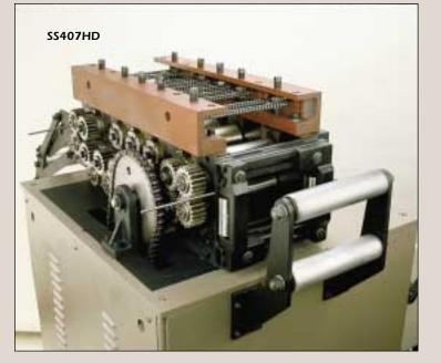
Robust best describes the construction and power of this series. Removal of coil set and curvature for thicker, wider materials requires larger diameter rolls and increase spacing.
