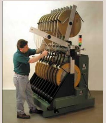
Loading of empty spools and removal of filled pancake spools are done by one operator. Interleaf material is loaded on a swiveldown holder assembly for easy set-up.
