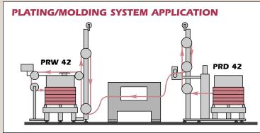
P/A's new Automatic Horizontal Systems are designed to **continuously** wind or rewind products directly to or from a palletized stack of multiple coils. By utilizing 40 inch reels it is possible to increase production by 40 to 80 percent.
