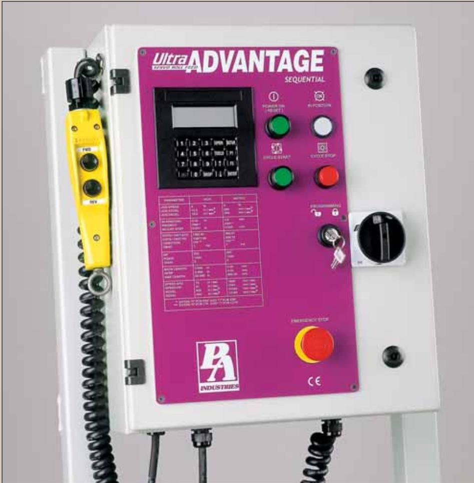
Another P/A innovation is the new sequential control for all Edge, Advantage, Magnum and Maximus models. The sequential software that provides the ability for step feeding, tool signaling, gagging and multiple programs off of one press or punching machine easily obtains flexible manufacturing using simple tools. Feed-to-registration capability is another design feature.
