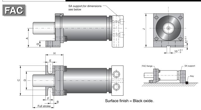
The FAC is a 90° angled, 2-piece flange for TU 750-5000 and TB 750-3000 gas springs. The flange is only to be used together with support SA or other support that supports the bottom of the spring. It is recommended the SA-mount is backed with a key, see figure above.
