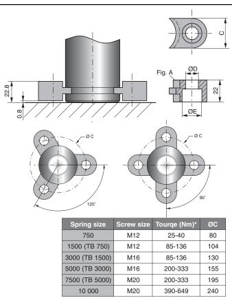
\*) Torque setting depends on the strength of screw used!
