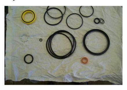
Lay out and grease all seals from seal kit. It is very important to grease the seals to avoid tearing during installation.
