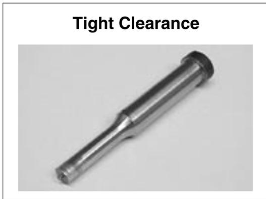
This example also illustrates the effects of tight clearance. The rings around the point indicate that the part material has sprung back on the point at snap-thru grabbing the end of the punch. This tight fit on the point has generated heat discoloring the area just behind the tip, potentially damaging its heat treat. Tool life due to heat damage will be reduced.
